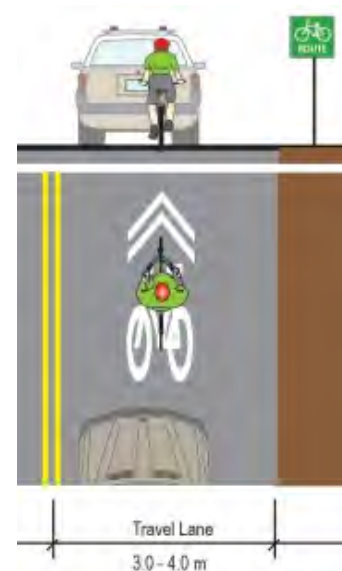
Signed Route on Local Road, Halton Hills, ON (Bottom Left) & Sample Signed-Only Cycling Route Cross Section with sharrow symbol; (Top) Source: MMM Group Signed Route on Local Road with Sharrow, Town of Carey (Bottom right); Source: townofcarey.org
