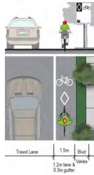
Sample Bike Lane Cross Section; (Top Right) Source: MMM Group Bike Lane on Local Road, Halton Hills, ON (Bottom Left); Source: MMM Group Bike Lane on Local Road, Holland; (Bottom Right) Source: www.wiki.coe.neu.edu
