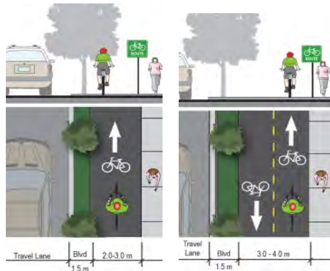
Sample Uni-Directional Multi-Use Path within the Road Right-of-Way Cross Section; (Top Left) Sample Bi-Directional Multi-Use Path within the Road Right-of-Way Cross Section; (Top Right) Source: MMM Group; Bi-directional Multi-use Path Example, Toronto, ON (Bottom Left) Source: MMM Group
