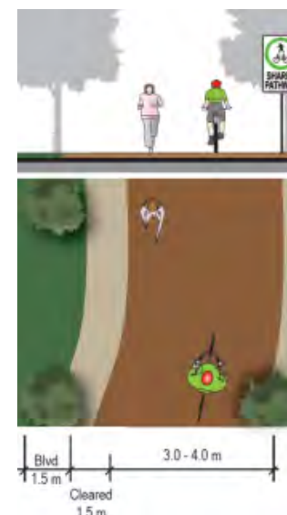
Off-Road Multi Use Trail, Stratford ON (Top Left); Source: MMM Group Off-Road Multi-Use Path Cross Section (Top Right) Source: MMM Group Paved Off-road Multi-use Trail, Ottawa Carleton Trailway (Bottom Left); Source: ontariotrails.on.ca
